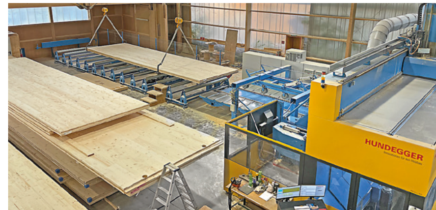
Elements measuring up to 3.6 by 16.5 m with a maximum thickness of 40 cm can be processed on the PBA-Drive
