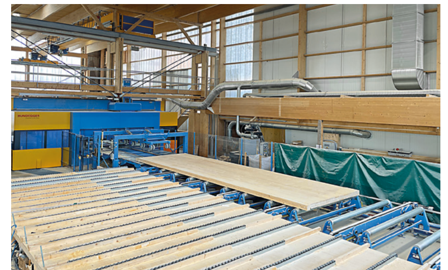
After the joining has been done, the CLT elements can be further finished on the cross conveyor
