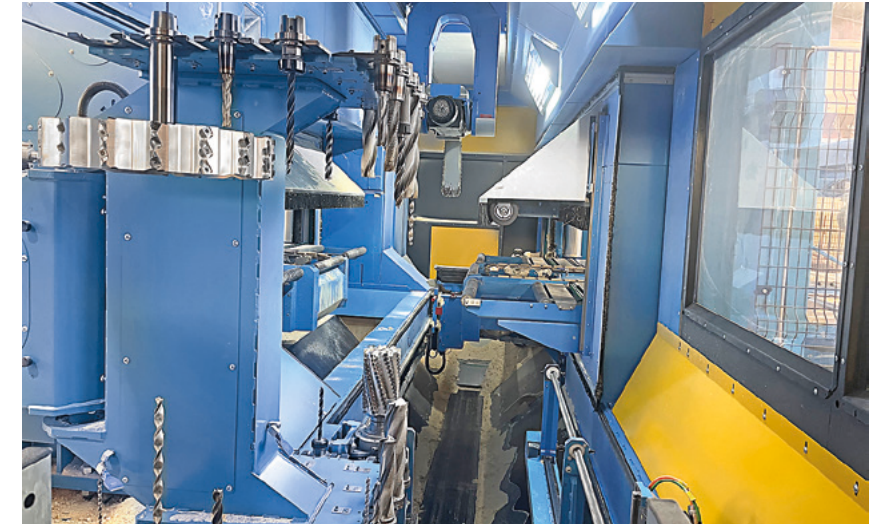
The tool magazine has space for 26 tools. The machine is also equipped with special tools, such as chain milling cutters and two deep-hole drilling units
