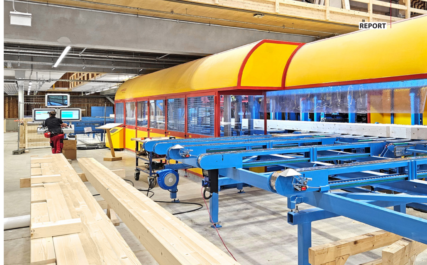
At Theurl, the automated infeed ensures the optimal utilization of Hundegger's K2-Industry machines
